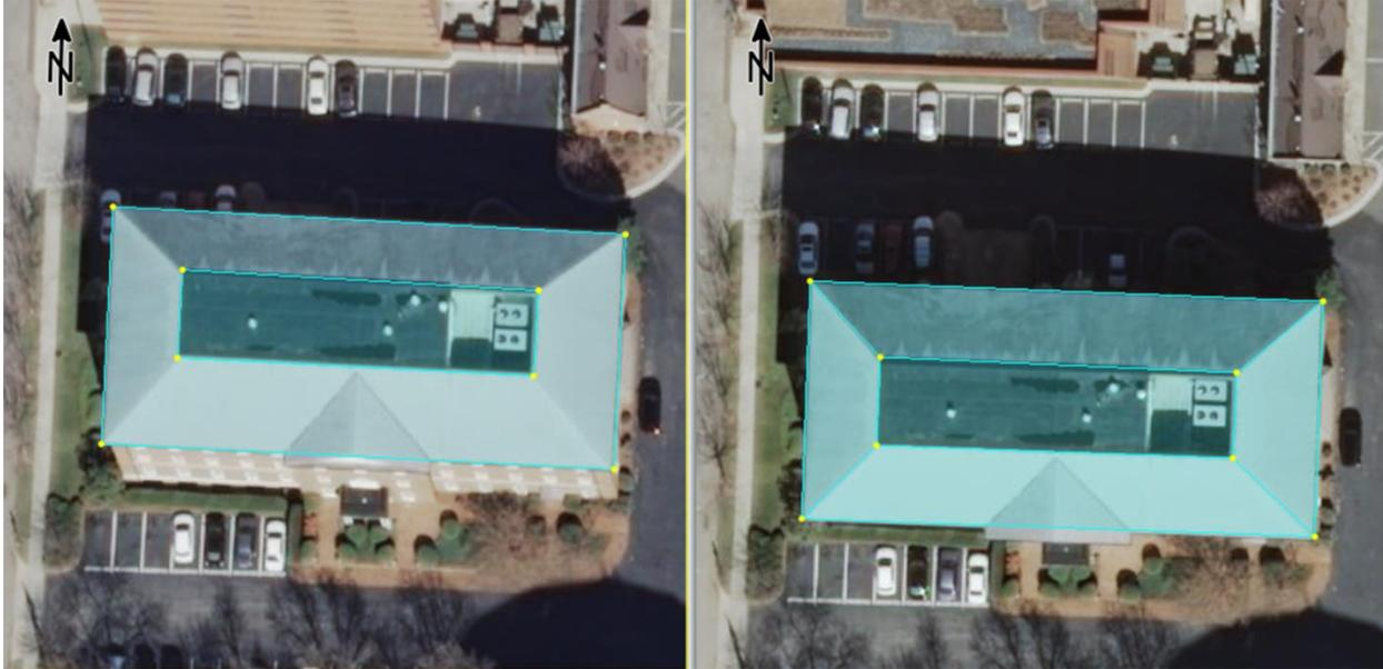
Figure 58. Loft a polygon to another polygon to create a truncated pyramid.
